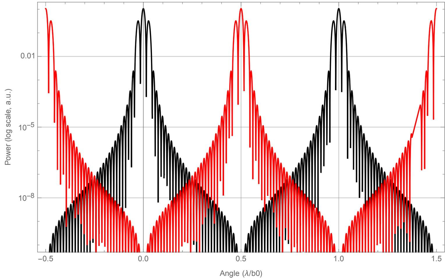
**Idea 2: Improvement with tailored coupling.** We can increase the suppression at the minimum, at the cost of broadening the main lobe, by *tapering*, ie selectively attenuating the incoming beams (akin to the PFB). The tapering pattern shown here produces the  $10^{-10}$  suppression/contrast we would need to separate the light from Earth versus the Sun.
