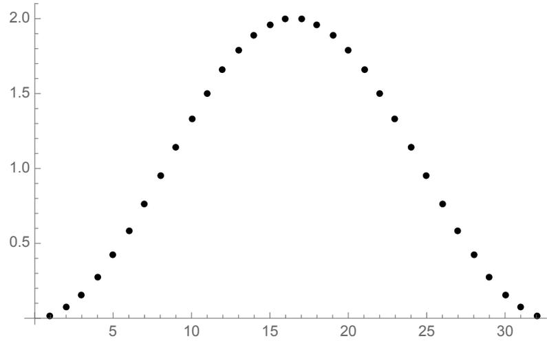
Tapered weighting pattern for each of 32 apertures. This is at the E field level, not the power level; so the same pattern but alternating in sign (below) applies to the alternating sum.
