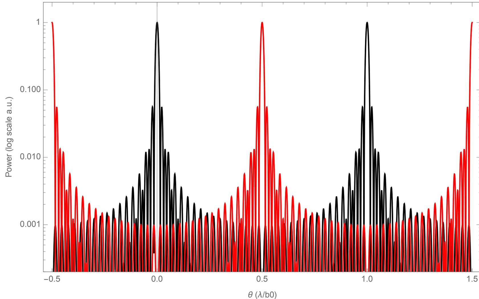
**Idea 1: Improvement with larger arrays.** We can improve the suppression of each beam in the area of its minimum by increasing the number of apertures; but only slowly. The beams for 32 apertures shown here have narrower main lobes but only a  $\sim 10^{-3}$  suppression near their minima.
