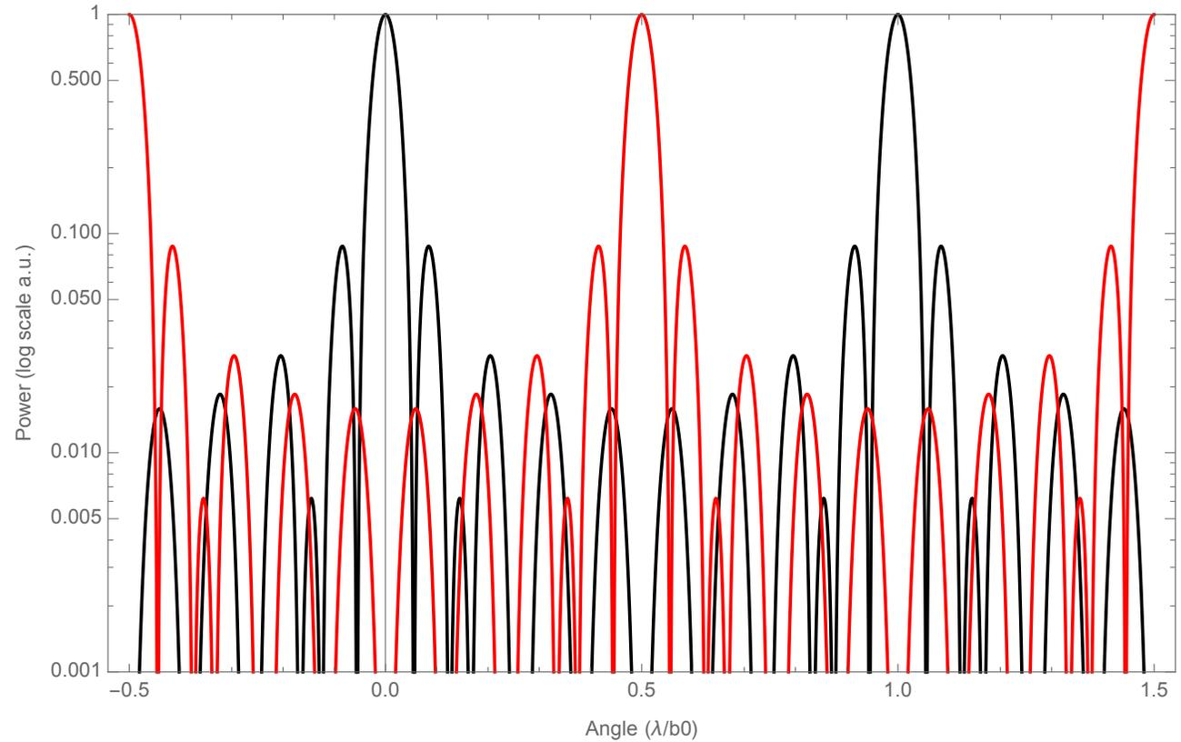
Plotting the power receptivity on a log scale allows us to see that, while one beam has a null where the other has a maximum the general level of the suppressed beam is on the order of 1/100.
