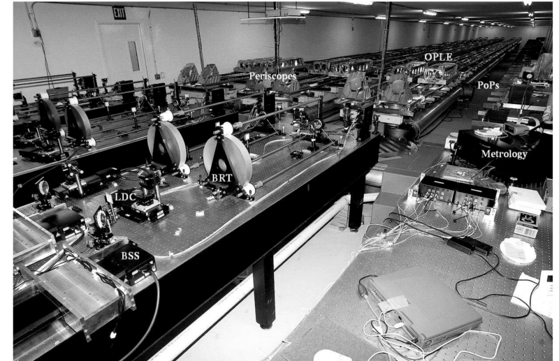
Beam line path length control at CHARA
